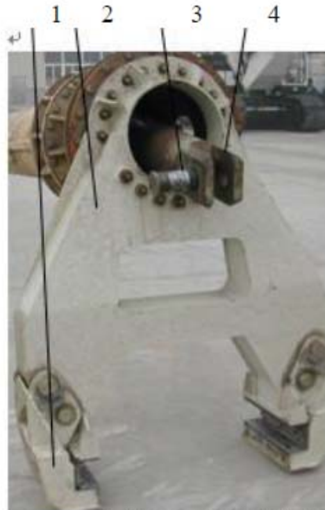
Fig.8-13 Placement of kelly bar to be Installed
