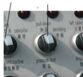
Fig.8-5 Switch of pull-down cylinder on the control panel
