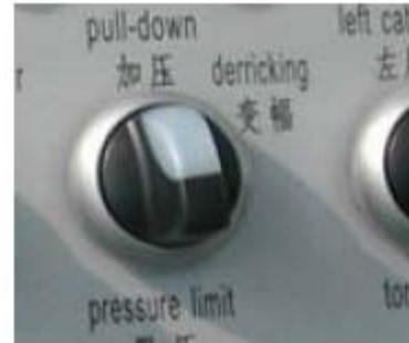
Fig. 5-9 Control switch of the pull-down cylinder
