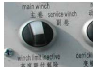
Fig. 8-10 Operation of main winch
