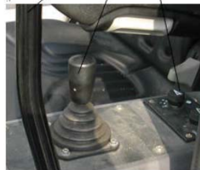
Fig.8-4 Control handle of mast lifting cylinder (mast) and A/C switch
