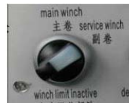
Fig. 8-11 Operation of service winch
