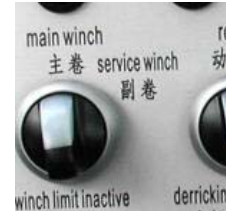
Fig. 5-7 Controlling main winch
